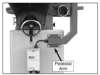
**Figure 12.** Correctly installed switch components.
